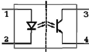
Schematic diagram of an opto-isolator showing source of light (LED) on the left, dielectric barrier in the center, and sensor (phototransistor) on the right.
