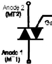
On the TRIAC symbol there are three terminals. These are the Gate and two other terminals. These other TRIAC terminals are often referred to as an "Anode" or "Main Terminal". As the TRIAC has two of these they are labelled either Anode 1 and Anode 2 or Main Terminal, MT1 and MT2.
