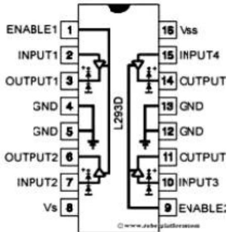
The Enable and Input pins are connected to Arduino pins. The Enable pins are connected to PWM enabled pins while the Input pins are connected to digital pins.
